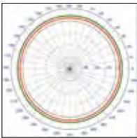
Signal Patterns 301127, 301143, 301149 Omni-directional when mounted vertically H - Plane @ 850 MHz H - Plane @ 1920 MHz
